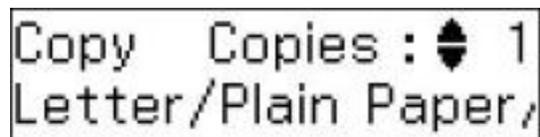
4. To print more than one copy, press the up or down arrow buttons to select the number (up to 99).
