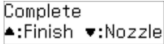
5. Press the down arrow to run a nozzle check and confirm that the print head is clean.
