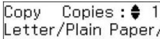
3. To print more than one copy, press the up or down arrow buttons to select the number (up to 99).
